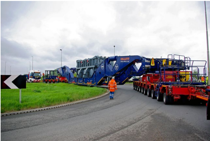
Image of a transformer being delivered to site on the abnormal indivisible load (AIL) vehicle.
